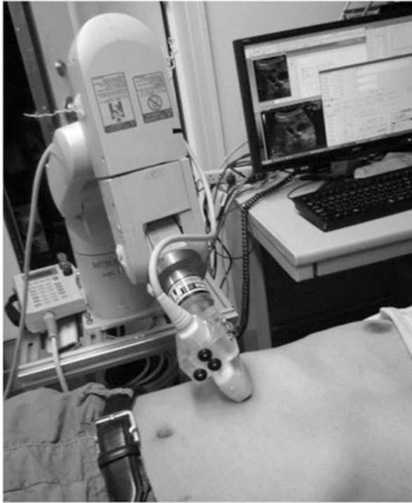
Fig. 2.5 Experimental setup of the liver tracking
