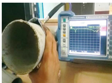
Fig. 10 Antenna under bending on 11 cm dia PVC pipe
