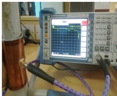
Fig. 9 Flexible software antenna placed on PVC pipe
