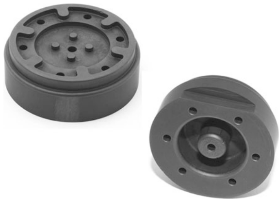
Fig. 3 ED-machined ZTA–TiC mold insert for injection molding, diameter 40 mm [13]
