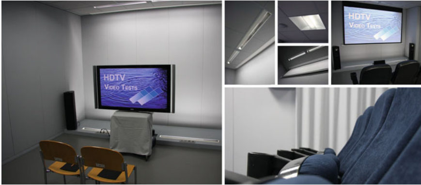
Fig. 2.3 ITU-R BT.500 compliant subjective testing laboratory at TUM: controlled lighting, colour-neutral mid-grey background, adaptability to different displays and test setups
