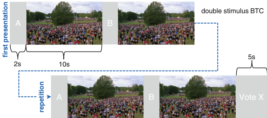
Fig. 2.7 Double stimulus BTC: presentation of reference A and test condition B , repeated once and then followed by a voting block
