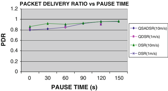
Fig. 4 Packet delivery ratio versus pause for Scenario 1
