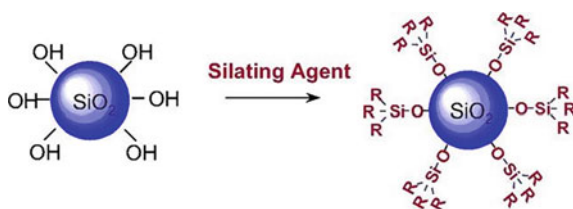
Fig. 2.4 Silylation process of silica aerogel (Soleimani Dorcheh and Abbasi 2008)
