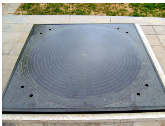
Fig. 2.36 The Direction Determining Board is a device used for establishing directional orientation. Invented by Guo Shoujing (1231–1316), the device was originally of wooden construction, but in later times copper was used instead. The square board measures four chi to a side. Source Photograph by Changsong Wang. Note Chi, cun and zhang are traditional Ancient Chinese units of length. 1 m \approx 3 chi, 1 m \approx 0.3 zhang, 3.33 cm \approx 1 cun.
