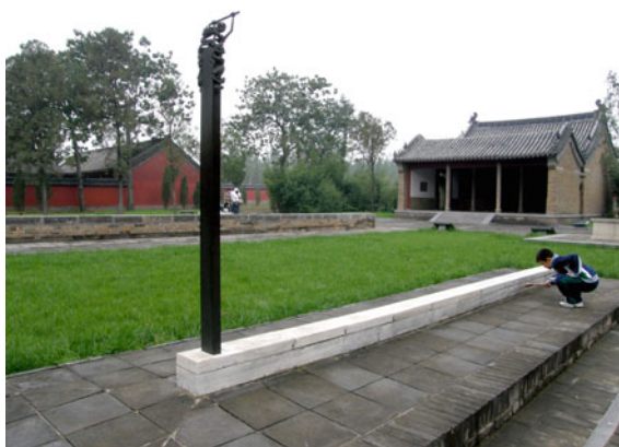
Fig. 2.38 A scaled-down replica of the Tall Ruler. This replica is one-fifth the size of the original. In most of the 27 observation stations in the early Yuan Dynasty (1271–1368), the Tall Rulers measure eight chi long; only the ones of the observatories in Beijing and Gaocheng measure four zhang long. Source Photograph by Ying Li
