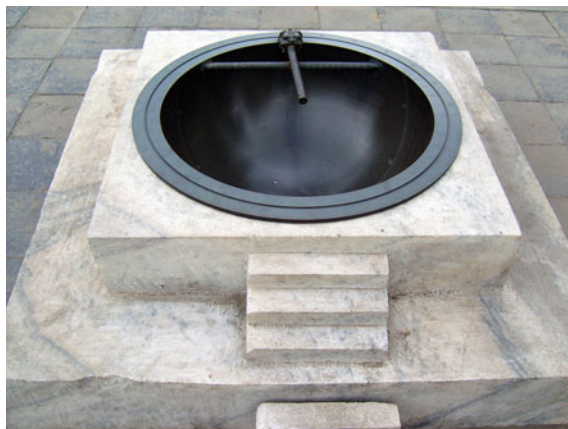
Fig. 2.37 This Scaphe is a one-fourth-scale replica of the original created by Guo Shoujing (1231–1316). It is actually a spherical sundial composed of an upward-looking cauldron, two crosses, and a silhouette aspheric board. The device was used to determine the sun's spherical location; it could also be used to measure solar displacement throughout the year and observe solar eclipses. Source Photograph by Changsong Wang
