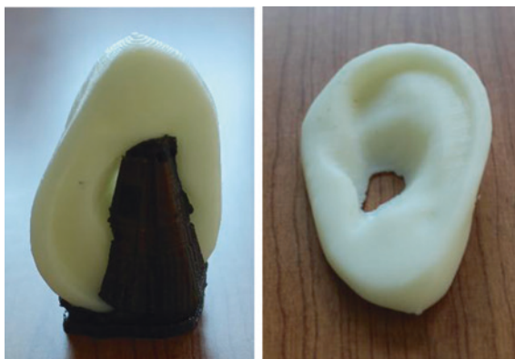
Fig. 2 Physical part with its support material before and after the removal process
