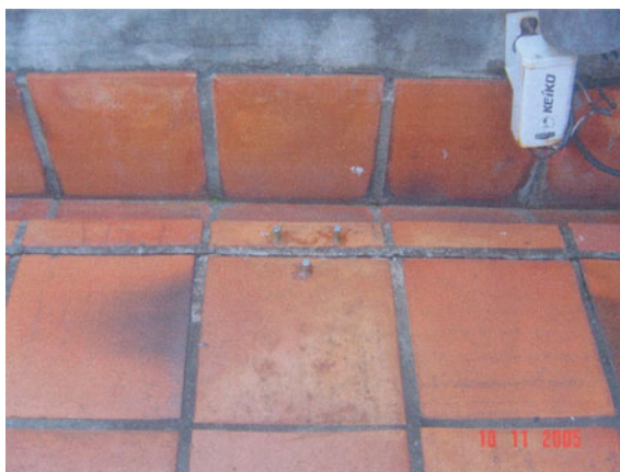
Fig. 17 Monitoring station and pins fixed to the south terrace, fifth floor (Nov 2005 —Cerne Engenharia)
