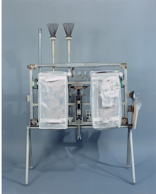
Fig. 2.9 The opposite side of the large tool carrier could accept two large lunar sample bags. (NASA)
