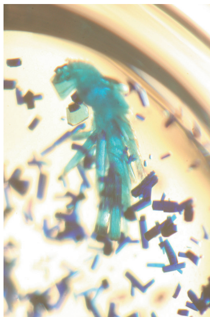
Fig. 5 In this vapor diffusion droplet containing sodium nitrate and a trace amount of sodium chloride, the protein lysozyme has crystallized in two distinctly different crystal forms. The large cluster of thin laths is the monoclinic crystal form, while the many smaller, darker crystals are of tetragonal symmetry
