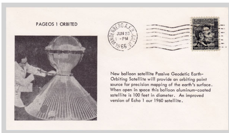
Fig. 2.17 PAGEOS 1 was a 30-m-diameter sphere made from 1.27 \mu\text{m} Mylar externally coated with a 0.22 \mu\text{m} vapor-deposited aluminum weighing 54 kg. The
