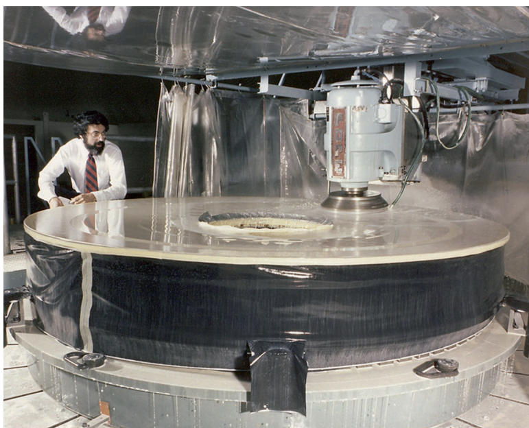
FIG. 2.2 HST's mirror blank being ground (Image credit: NASA)
