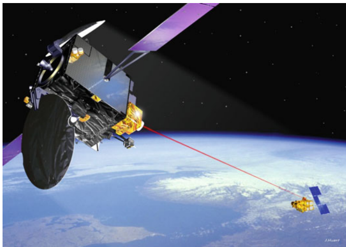
Fig. 2.40 ISL of GEO spacecraft Artemis—Courtesy of Webpage: by ESA
