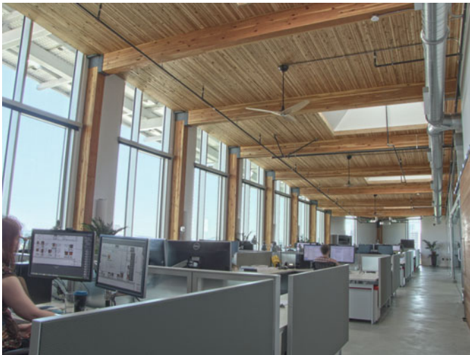
Fig. 2.4 Sixth floor daylight perimeter zone. Note the absence of a conventional installation of electrical lighting fixtures on the ceiling
