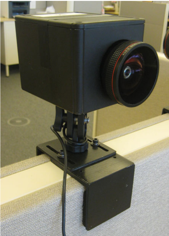
Fig. 2.28 Field installation of High Dynamic Range (HDR) enabled camera for acquisition of time-series measurements
