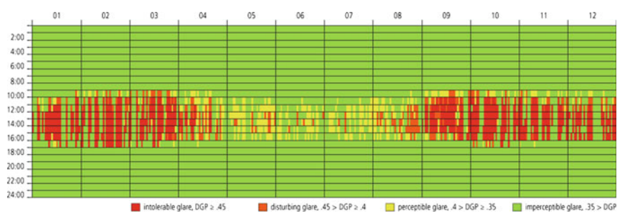
Fig. 2.33 Annual Daylight Glare Probability (DGP) simulation. The x-axis corresponds to 365 days of the year, the y-axis corresponds to time of day. Red and orange fields correspond to hours with intolerable or disturbing glare, respectively, yellow to perceptible glare and green to imperceptible. Image credit Alstan Jakubiec
