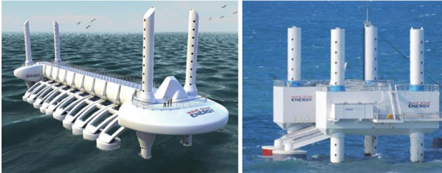
Fig. 2.21 Wavestar prototype with two floaters, at DanWEC, Hanstholm, Denmark ( left ) and concept for full scale deployment, artists impression ( right ). Courtesy of Wavestar [38]
