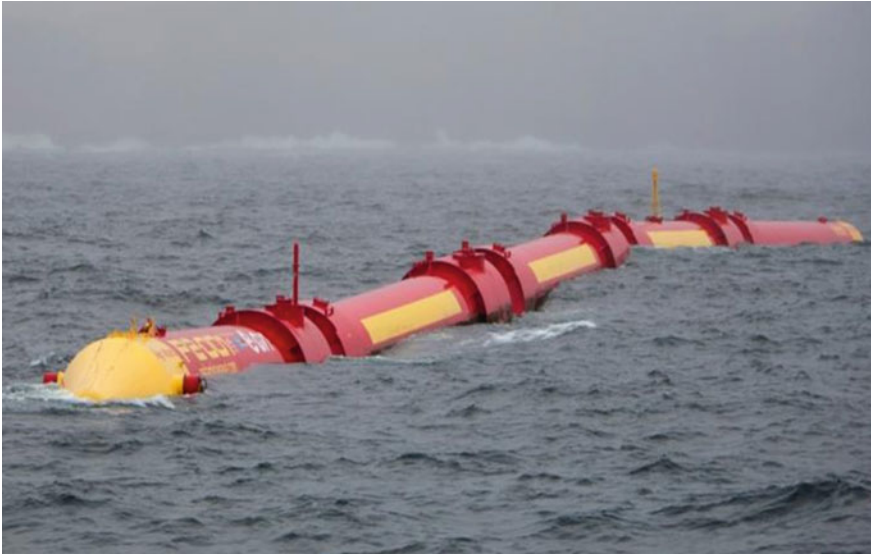
Fig. 2.9 E.ON P2 Pelamis operating in Orkney July 2011 [27]
