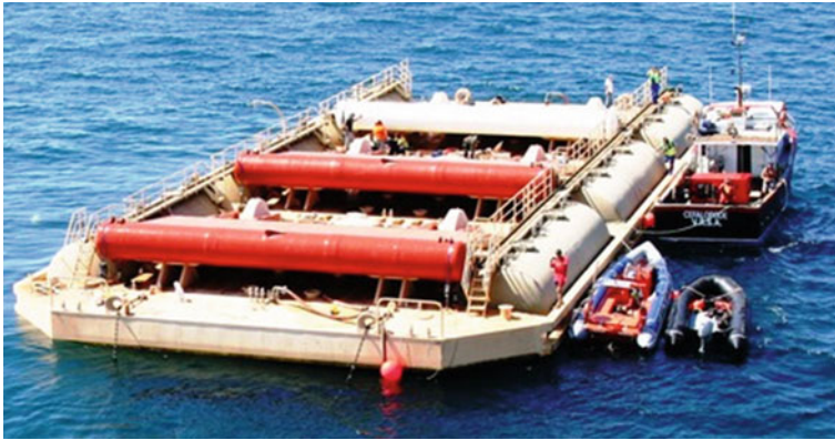
Fig. 2.18 Waveroller WEC prototype, before submerged to seabed [35]
