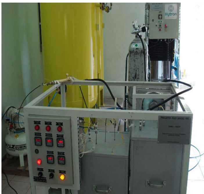
Fig. 2.20 Steam reforming of ethanol prototype: catalyst reduction
