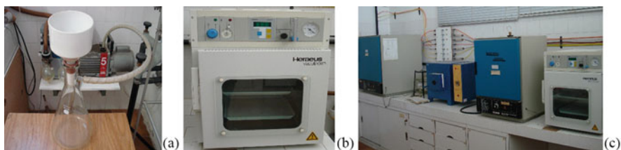
Fig. 2.13 Equipments utilized: (a) Washing-filtration, (b) vacuum drying, and (c) calcination systems
