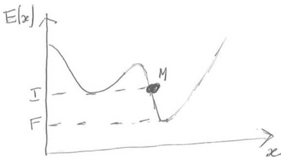
Fig. 2.1 Potential energy E = Mgh and the evolution of a mechanical system
