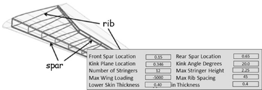
Fig. 2.16 Spars and ribs dimensioned automatically by the KBE engine
