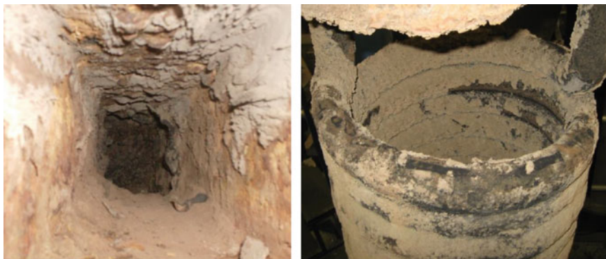
Fig. 2.10 Left Fly ash deposits ( slagging ) in a plant duct. Right condensation of alkali components on the chilling unit ( fouling )
