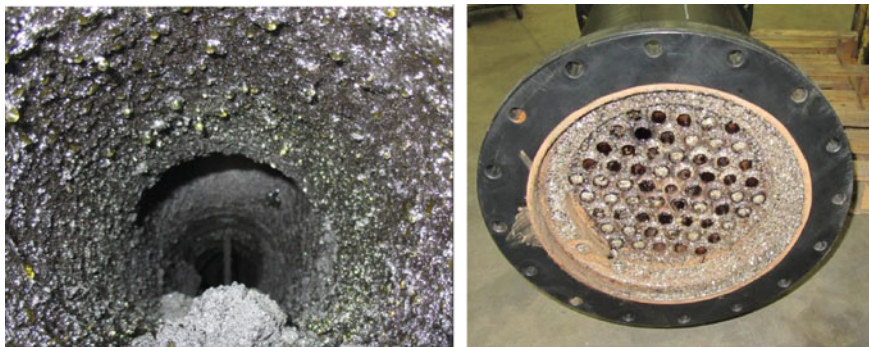
Fig. 2.11 Tar condensation ( left ) and crystals build-up ( right ) on heat transfer surfaces
