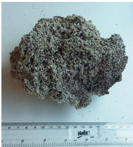
Fig. 2.9 Large agglomerate formed from RDF ash sintered and sand particles
