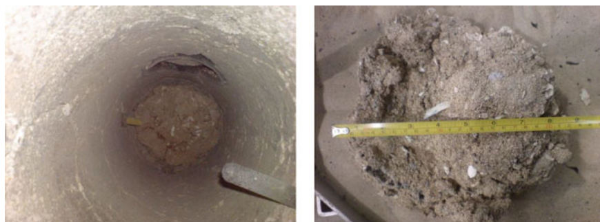
Fig. 2.7 Fused bed in FBG ( left ) and closer inspection of fused pan ( right )
