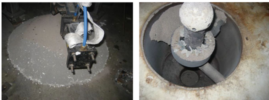
Fig. 2.5 Left Dry discharged bed ( bottom ash ) from FBG showing plenty of bones and stones and right presence of glass fraction on the fluidising nozzle
