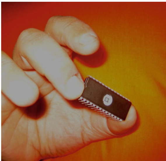
Fig. 1 EPROM device with the silicon window that enabled erasure by UV
