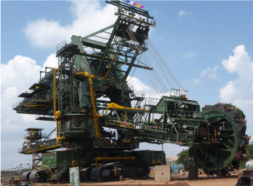
Fig. 2.3 C-frame bucket-wheel excavator—BWE700L
