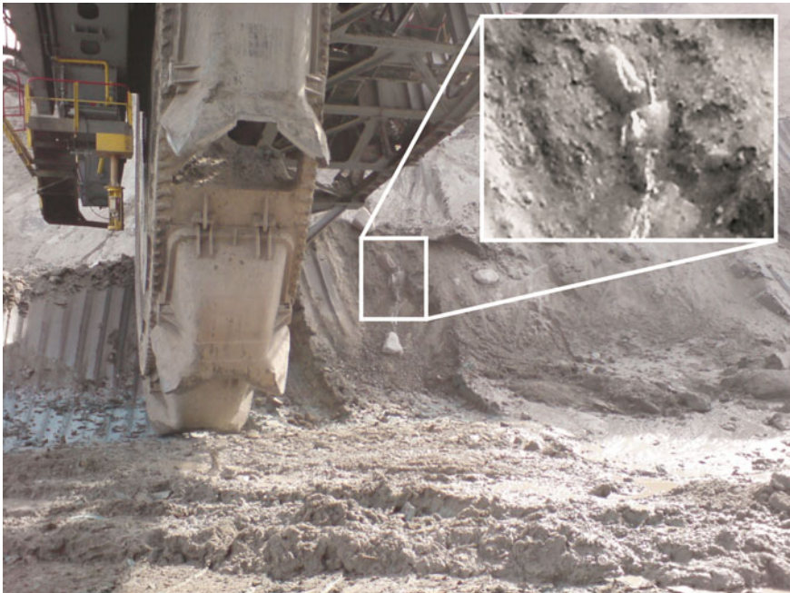
Fig. 2.31 Overburden with non-mineable formations in a surface mine
