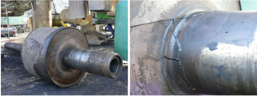
Fig. 2.15 Damage to the bucket-wheel drive shaft in the KWK 1200M excavator
