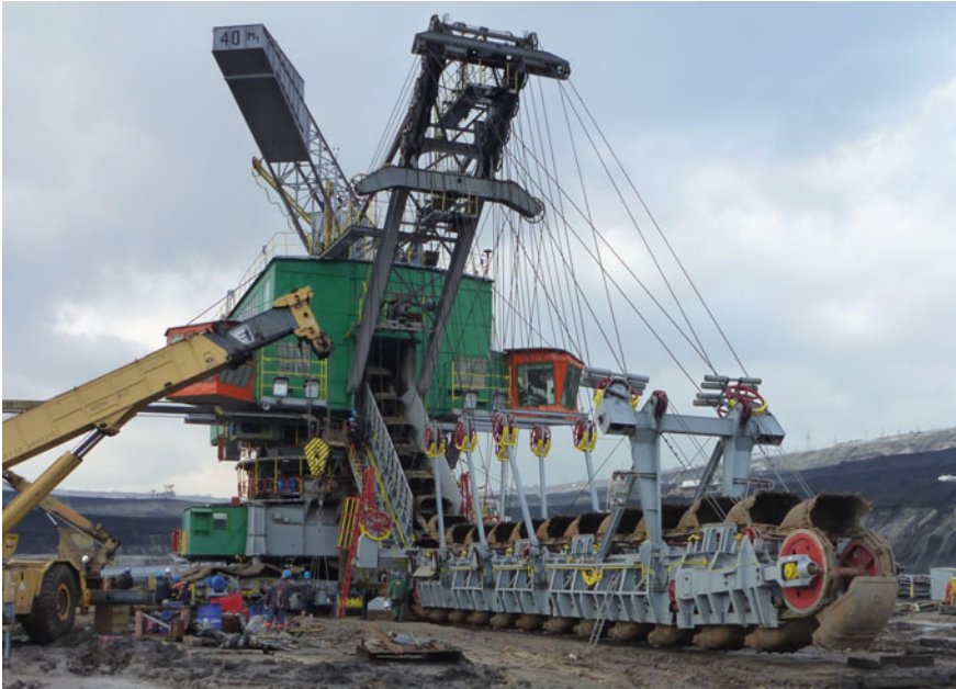
Fig. 2.10 Multibucket chain excavator—ERs710
