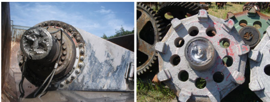
Fig. 2.20 Examples of damage to the drive trains of tracked undercarriages
