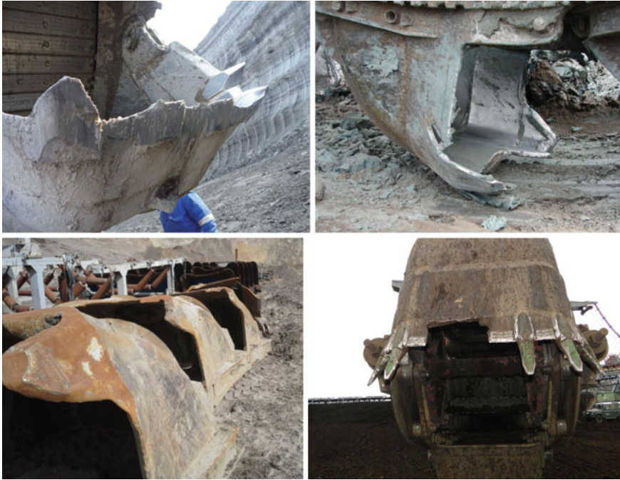
Fig. 2.17 Wear and damage process of buckets
