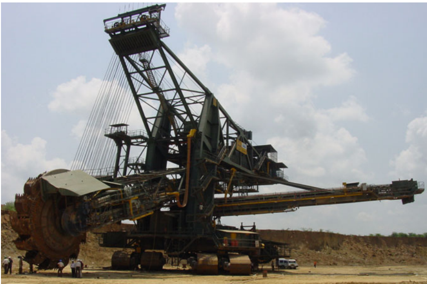
Fig. 2.4 C-frame bucket-wheel excavator—BWE1400L
