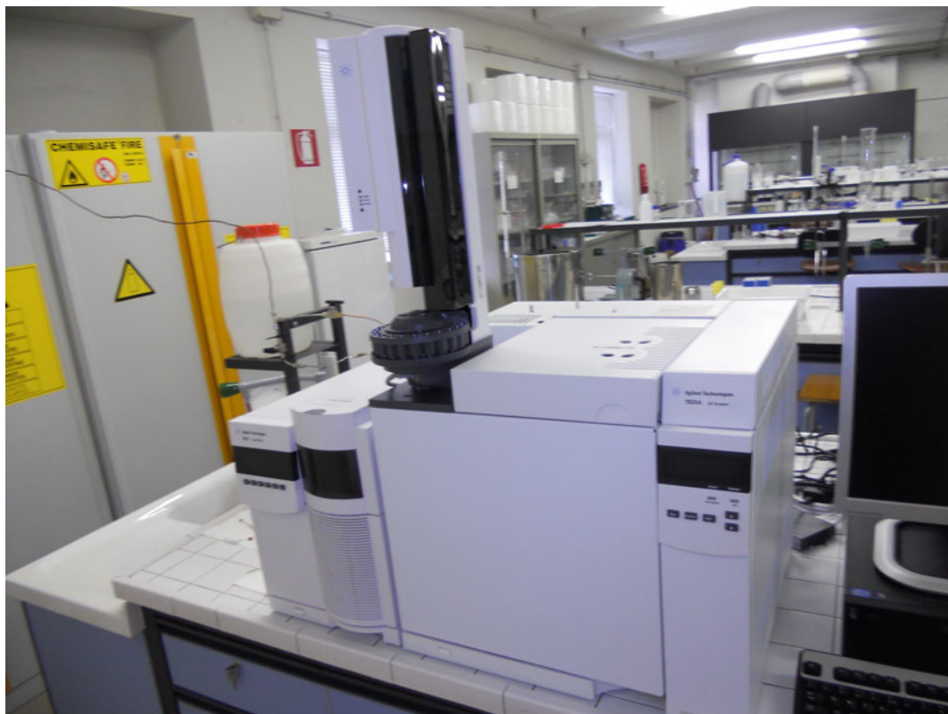
Fig. 7 A GC-MS system in a metabolomics laboratory
