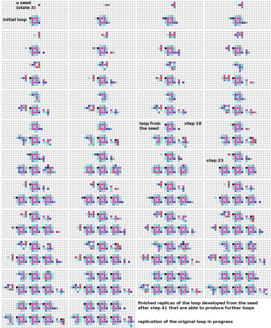
Fig. 9. A sequence of CA steps demonstrating the parallel replication of the small loop according to the evolved transition function from Fig. 10. The states are ordered from left to right and top to bottom. The bottom part of each state shows the replication from the initial loop, the top part of each state demonstrates the development and replication of the loop from a seed.
