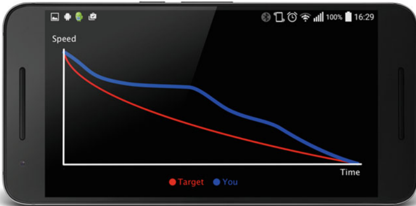
Fig. 2.1 Sample target curve (red) and braking performance (blue) shown in the prototype implementation
