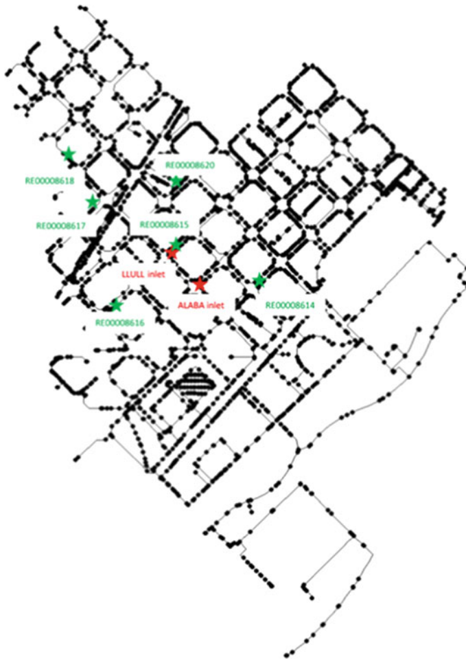
Fig. 2.8 Nova Icària DMA. In red , the two inflows, (flow and pressure sensors) and in green , the inner pressure sensors
