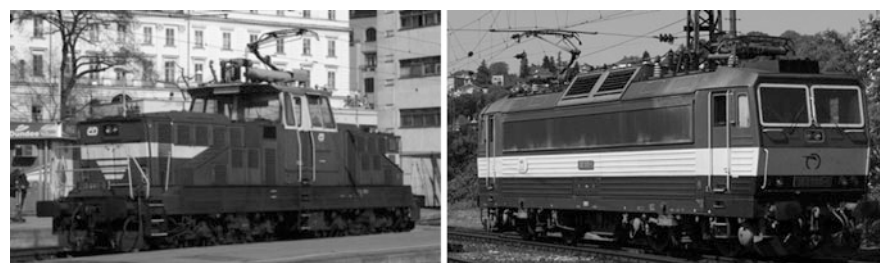
Fig. 3 Locomotive type 210 with a thyristor controller and uncontrolled rectifier, ( \text{DPF} \cong 0.76 ) and locomotive type 362 with an input converter filter, ( \text{DPF} \cong 0.87 )
