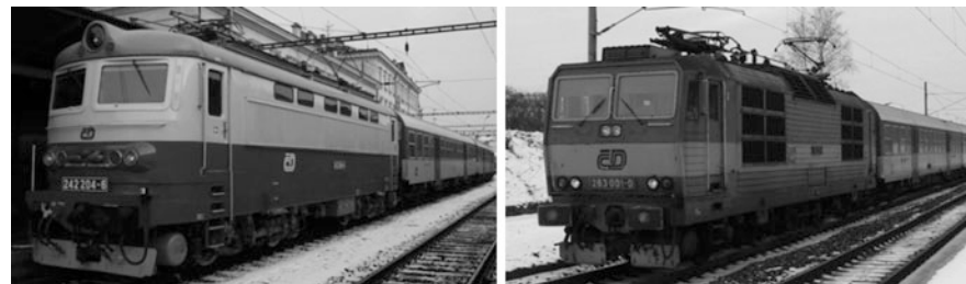
Fig. 2 Locomotive type 242 with a diode rectifier, ( \text{DPF} \cong 0.84 ) and locomotive type 263 with a thyristor-diode bridge, ( \text{DPF} \cong 0.77 )
