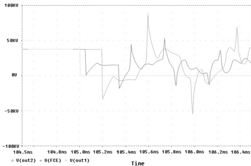
Fig. 22 The voltage at traction substation and the voltage at the end of the catenary A after short-circuit at the end of the catenary B
