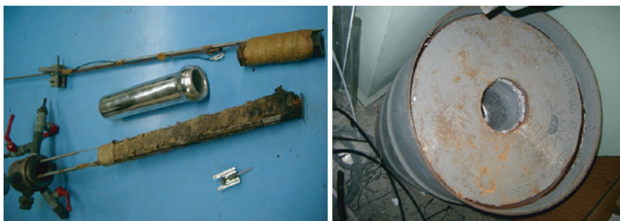
Fig. 2.3 Superconductivity in high tropicality conditions (HTC). Left panel Home-made inserts to perform transport measurements in superconducting samples at liquid nitrogen temperature and above. The mummy-like stick at the bottom includes a long cooper coil (wrapped in masking tape) to apply a magnetic field to the sample, while it is positioned at different heights inside a liquid nitrogen reservoir—a simple way to control the sample’s temperature without loss of homogeneity in the applied magnetic field. Right panel A magnetic shield to do measurements using a superconductor-based sensitive detector of magnetic fields (SQUID). The handwritten “brand name” reads “Tropical SQUIDS, Inc.” All these devices were made back in the early 1990s
