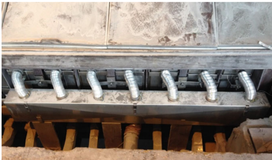
Fig. 7 EnPot heat exchanger units fitted on one sidewall of an aluminium smelting pot, connected to ducting for hot gas extraction, figure reproduced from [4]
