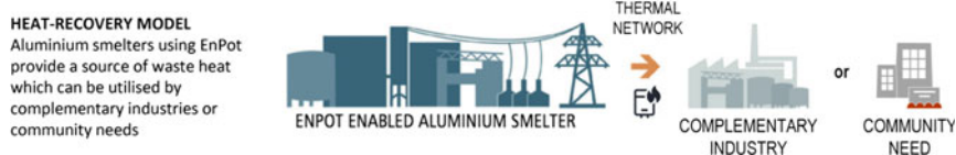
Fig. 10 Potential future model of smelter-industry/community relationships recovering heat from EnPot technology to complement surrounding industries or heating needs in the community
