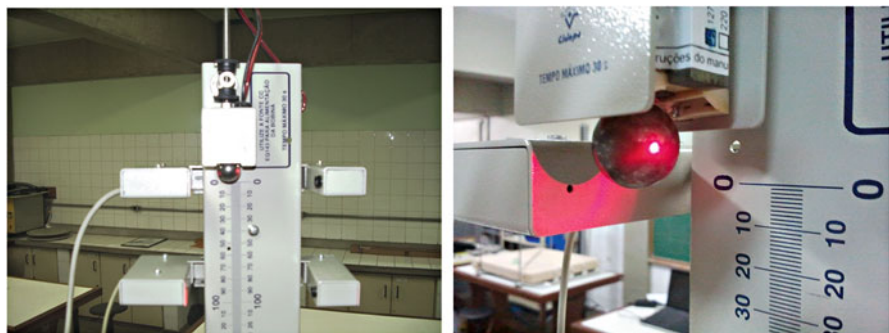
Fig. 2.2 Initial position of the metallic sphere. It is important to align the lower part of the sphere as close as possible to the zero position. This means that the lower part of the sphere's shadow should be as close as possible to the photosensor's aperture at the imminence of the start of the experiment (the photosensor emits an electronic signal when the laser is blocked by the sphere)
