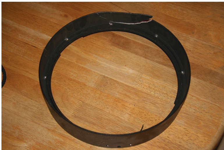
Fig. 2 The cracked Schmidt corrector plate cell
