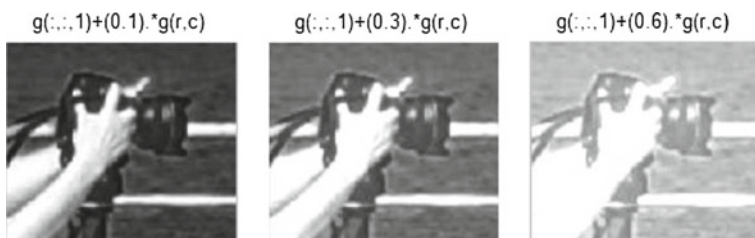
Fig. 2.16 Internal greyscale view of max-modified red channel intensities
