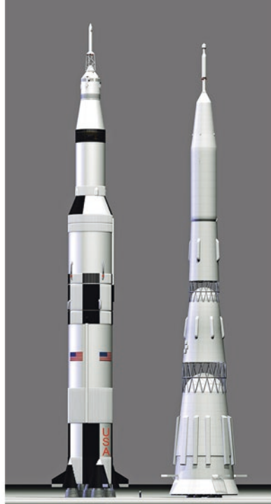
Comparison of NASA's Saturn V and the Soviet N1/L3. [Wikipedia Creative Commons/Ebs08]
