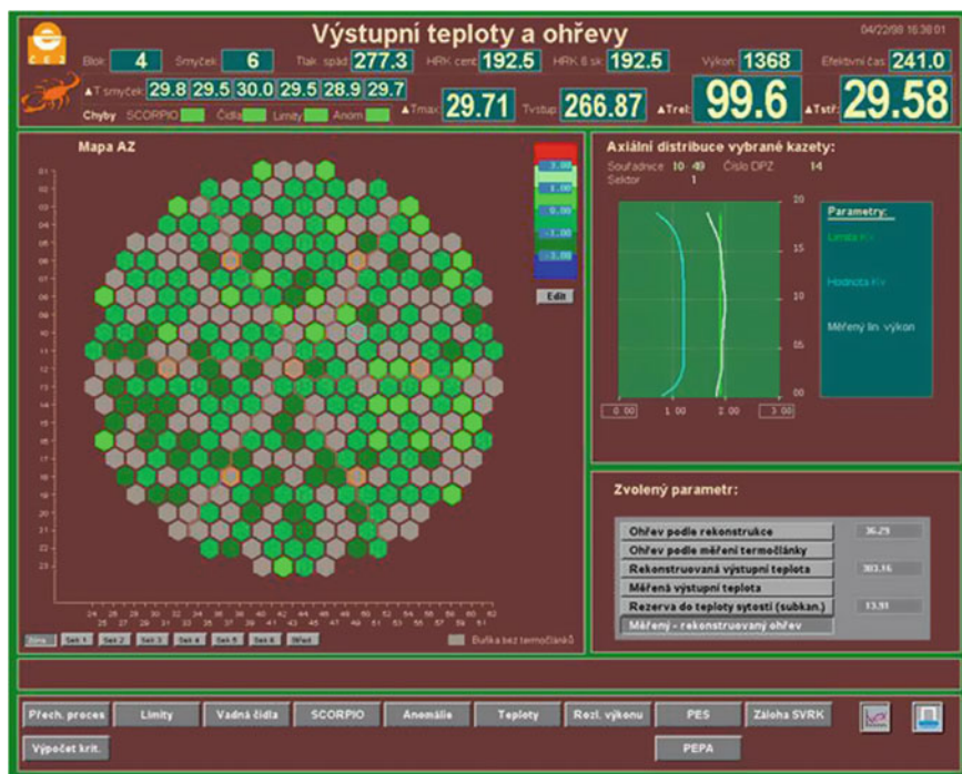
Fig. 2.39 An example of a core map picture in the SCORPIO-VVER system
