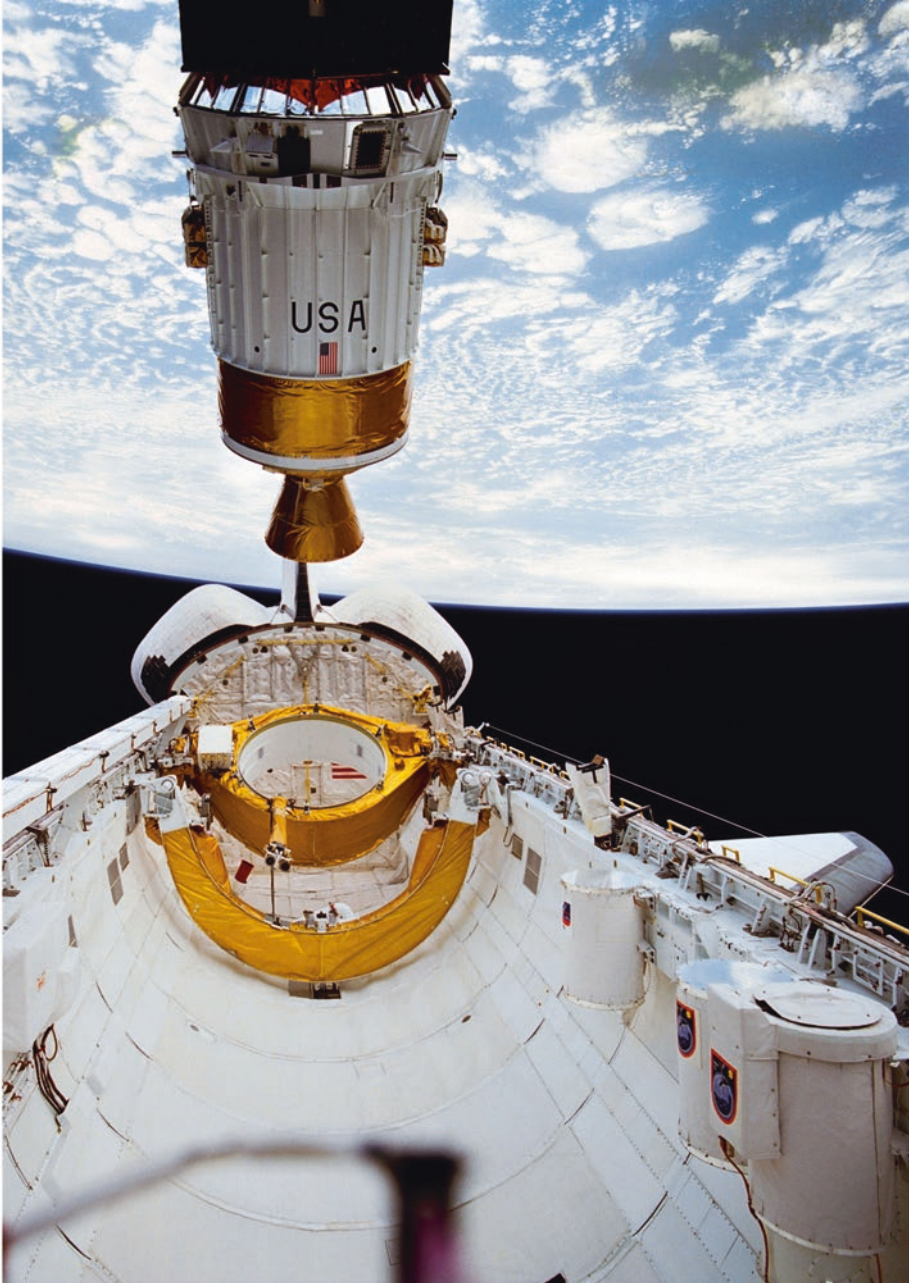
The Upper Inertial Stage and its payload begin their journey to geosynchronous orbit. Clearly visible in the background are the forward and aft frames of the airborne support equipment. Both are covered with gold-coated thermal insulation blankets.
