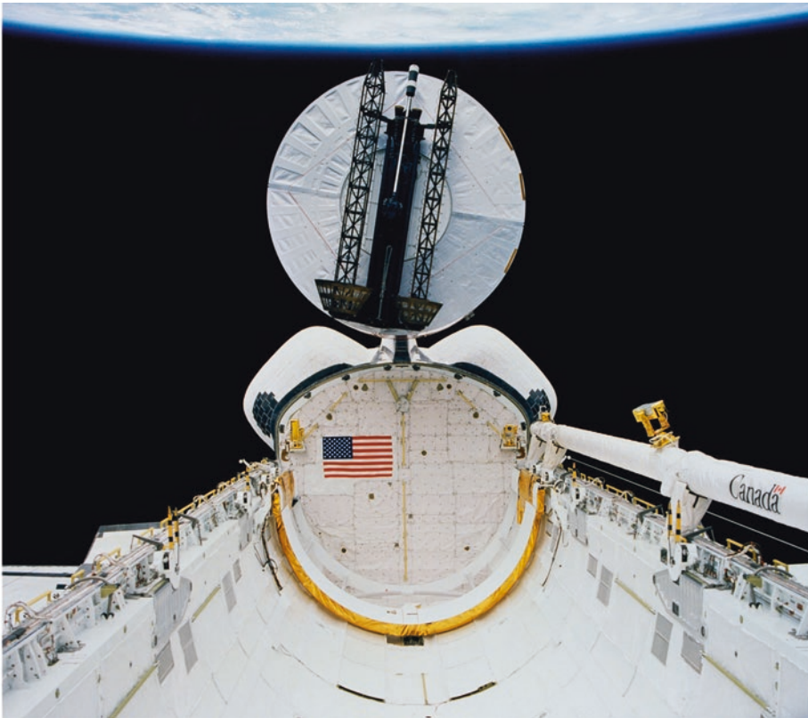
A Syncom satellite rolling out the payload bay. In the background is the cradle covered in a gold-coated insulating Mylar blanket.
