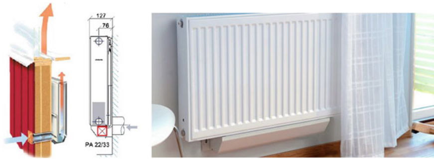
Fig. 2.6 Panel radiator operating in an integrated ventilation system [8]
