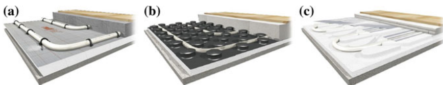
Fig. 2.16 An underfloor radiator made using the wet a, b and dry c technology [8]
