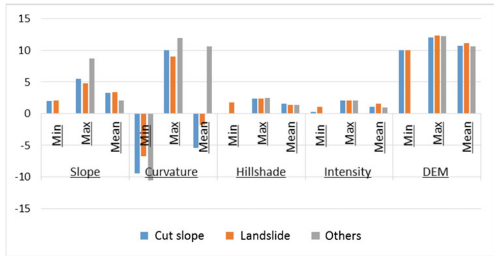
Fig. 2.19 Typical values of LiDAR-based features for landslide and non-landslide features. Note (1) slope \times 10 ; (2) hill shade, intensity, and DEM \times 102
