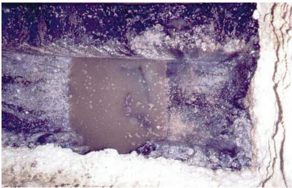
Fig. 2.2 Expanded residue of CaSO 4 on the concrete surface
