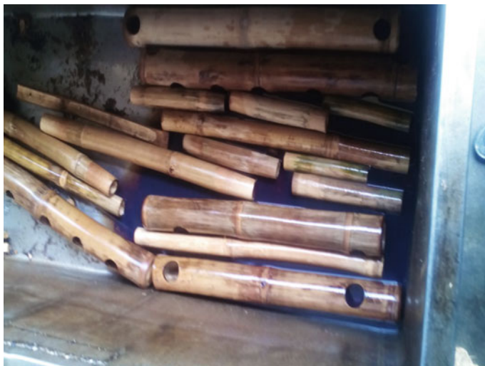
Fig. 2.10 Traditional Ghanaian method of preserving bamboo culms
