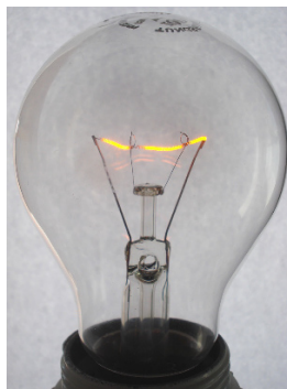
Figure 2.19: An incandescent light bulb emits visual, short wavelength radiation due to the high temperature of the filament, which is heated by an electric current.
