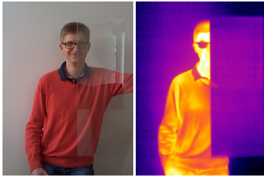
Figure 2.21: The same scene recorded by an optical camera (left) and an infrared camera (right). Because the glass transmits short wavelength (visual) radiation but does not transmit long wavelength (infrared) radiation, the infrared emitting objects are screened by the glass. Infrared thermography will be elaborated on in Section 2.4.4.
