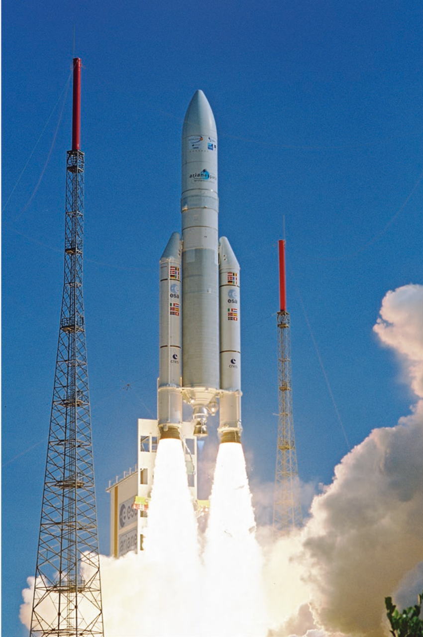
Figure 2.1: Ariane 5 flight V198. Ariane 5 is ESA's heavy lift launch vehicle that is part of the Ariane expendable launch system, capable of delivering payloads into geostationary transfer orbit or low Earth orbit. Operated and marketed by Arianespace, the rockets are launched from the Guiana Space Center in French Guiana. Originally designed to launch ESA's Hermes spaceplane, Ariane 5 was repurposed to launch satellites after the spaceplane idea was dropped in 1992. Credit ESA
