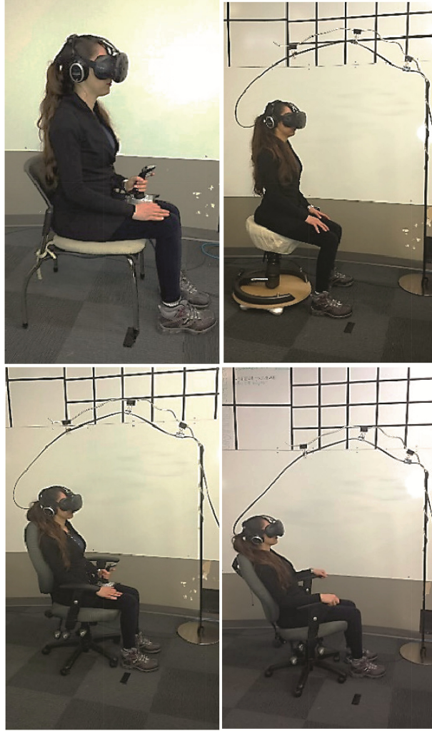
Fig. 2. Locomotion interfaces – (top-left) joystick, (top-right) NaviChair, (bottom-left) Real-Rotation, (bottom-right) Swivel-Chair
