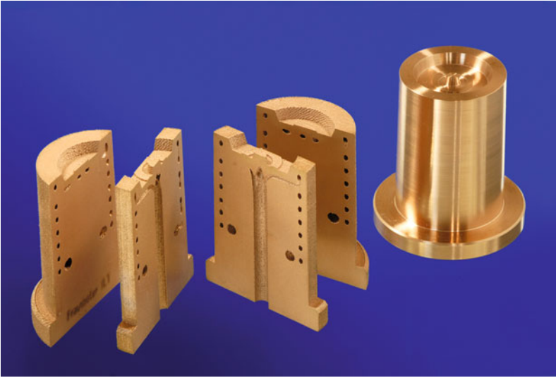
Fig. 2.27 Tool insert with internal cooling structures made from Hovadur K220 by SLM. 57
