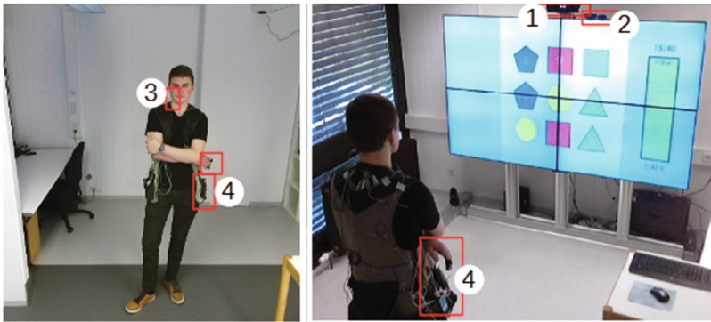
Fig. 2. Overview of the setting with sensors: (1) MS Kinect 2, (2) frontal webcam, (3) wireless headset, (4) GTec g.MOBILab+ biophysical sensor with sensors attached to the users body.
