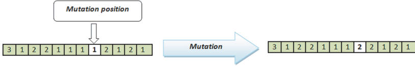
Fig. 3. Illustration of mutation operator
