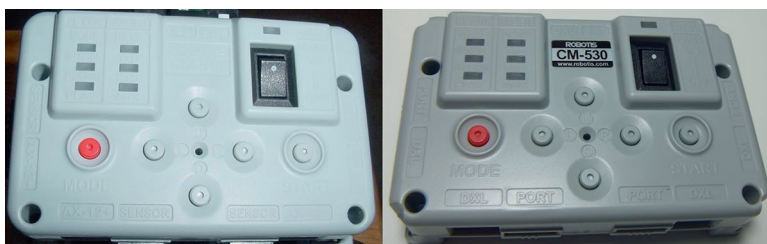
Fig. 2.14 CM-510 ( left-discontinued ) and CM-530 ( right ) controllers
