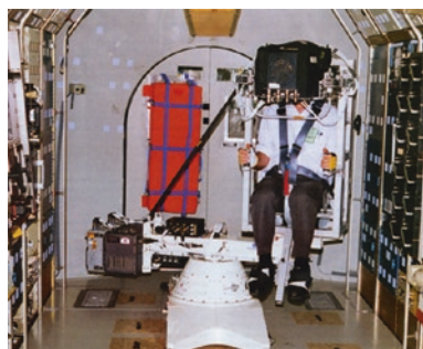
Fig. 2.2 The short-arm centrifuge employed for the tilt-translation experiment onboard the Shuttle seen here in the training mock-up (from Clément et al. 2001)
