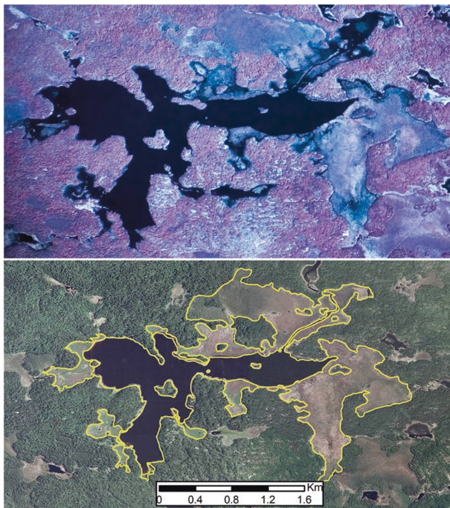
Fig. 2.11 The 2001 collapse of an outlet beaver dam reduced the impounded area of Shoepack Lake and adjacent wetlands from 366 ha in 1992 ( top ) to only 126 ha in 2003 ( bottom ). The yellow outline is the maximum extent of flooding
