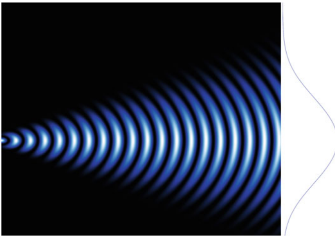
Fig. 2.3 The double-slit experiment with waves when only the lower slit is open. The intensity of the wave is shown in white (more intense) and blue (less intense). The blue curve on the right of the figure indicates the intensity of the wave on the second wall (A. Gondran cc by-sa 4.0)
