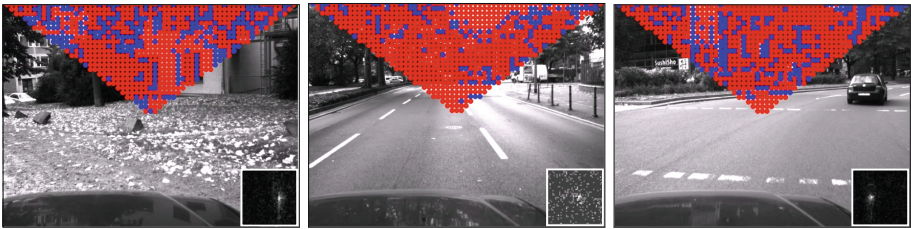
Fig. 5. Inferring current yaw rate: Car turns left (left) goes straight (middle) and (right) turns right. From pixels within the upper triangle the current yaw rate is to be inferred. At each time step only the pixels showing an event are taken into consideration, here marked blue. At each time step a mother accumulator is build by summing up all \Omega_{s_t} from which the current yaw rate can be inferred shown in the lower right part of every image. See text for details. (Color figure online)
