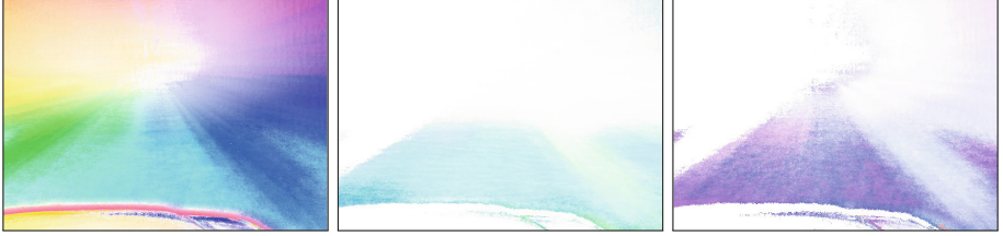
Fig. 2. Dense flow and confidence maps: for sequence GUCar after 50000 processed frames. (left) Colour coded dense flow map, (middle) eigen vector corresponding to the smaller and (right) larger eigenvalue of the accumulator’s covariance matrix. Colour encoding according to colour wheel (cf. Fig. 1). Best viewed in colour. (Color figure online)
